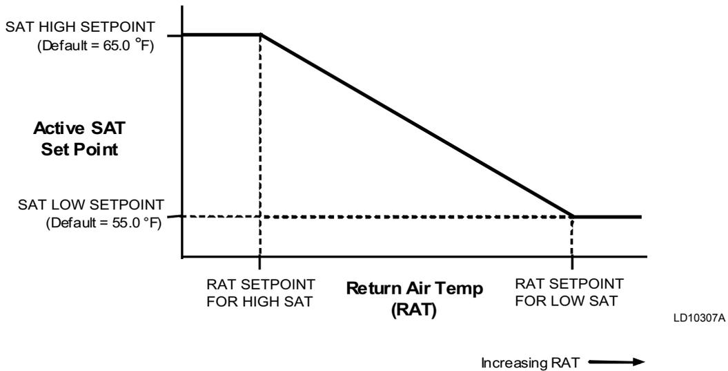
**FIGURE 34 - ACTIVE SAT SETPOINT VS. RETURN AIR TEMP**
