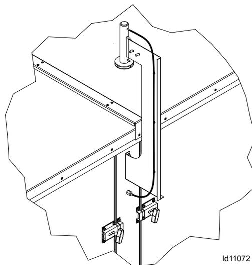
**FIGURE 17 - STATIC PRESSURE PROBE INSTALLATION**
