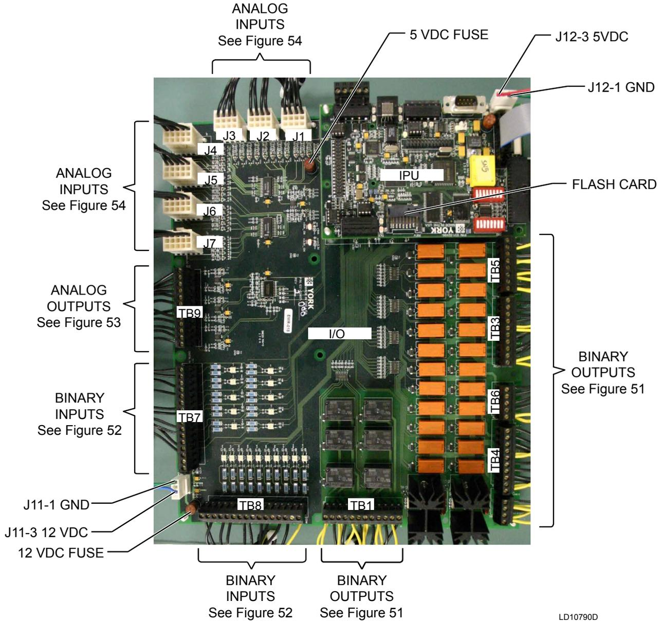
FIGURE 50 - I/O CONTROL BOARD
