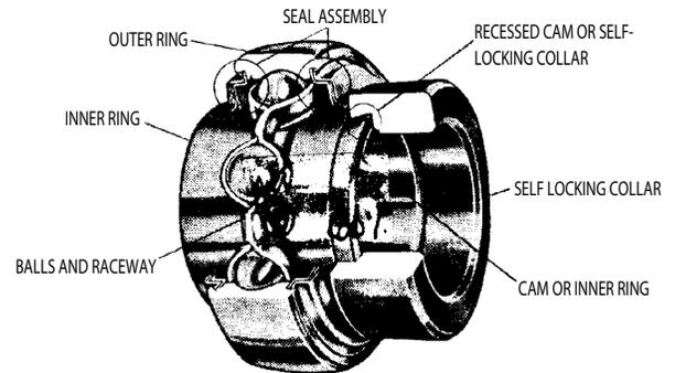
**FIGURE 26 - BEARING WITH ECCENTRIC CAM**
