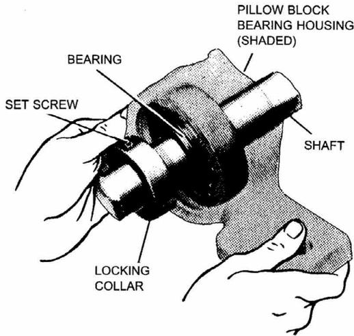
NOTE: Do Not apply excessive force to the bearing housing (pillow block or flange when installing the bearing on the shaft.
