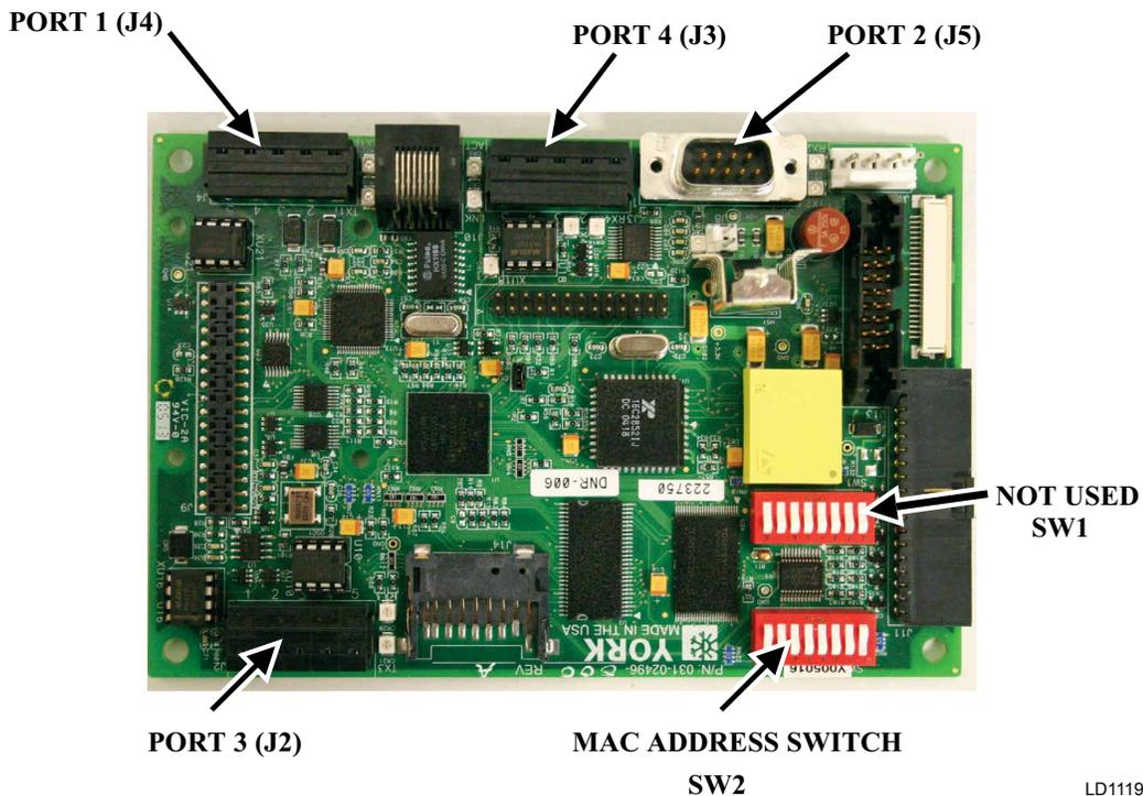
**FIGURE 48 - IPU CONTROL BOARD**
