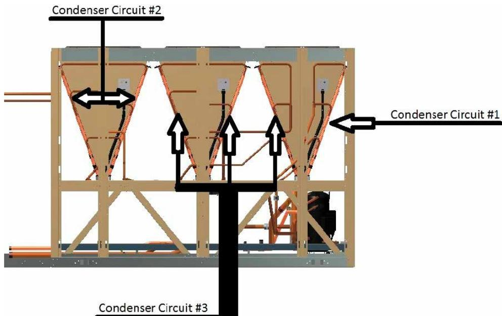
**FIGURE 37 - CONDENSER COIL IDENTIFICATION**
