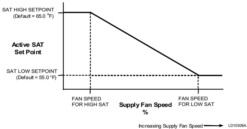
**FIGURE 35 - ACTIVE SAT SETPOINT VS. SUPPLY FAN SPEED**
