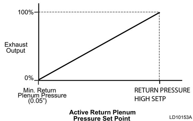
**FIGURE 46 - ACTIVE RETURN PLENUM PRESSURE SETPOINT VS. EXHAUST OUTPUT.**
