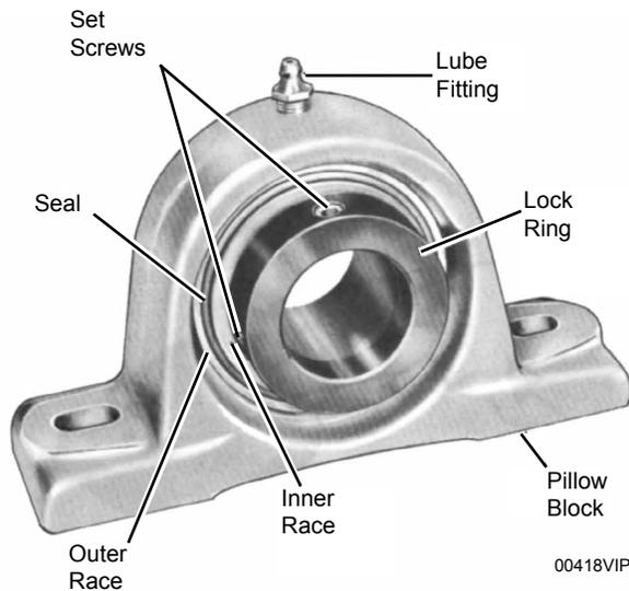
**FIGURE 25 - BEARING WITH SETSCREW TYPE LOCKING DEVICE**
