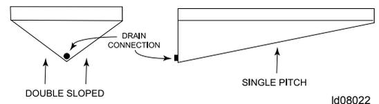
**FIGURE 2 - DOUBLE SLOPED SS DRAIN PAN**
