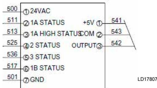
**FIGURE 40 - DIGITAL MULTIPLEXOR CONNECTIONS - MODULATING GAS HEAT**
