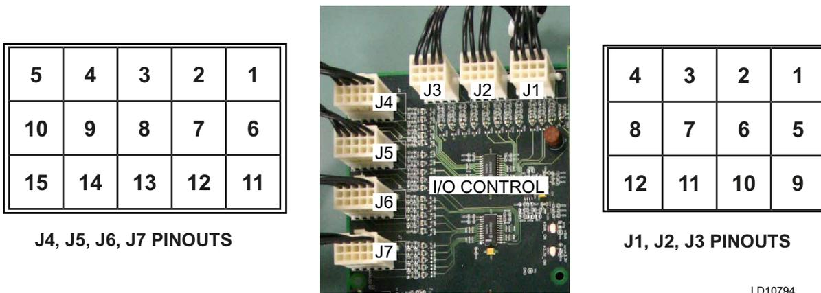
FIGURE 54 - I/O CONTROL BOARD - ANALOG INPUTS (SEE TABLE 61 ON PAGE 189 FOR PIN OUTS)
