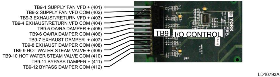
FIGURE 53 - I/O CONTROL BOARD - ANALOG OUTPUTS
