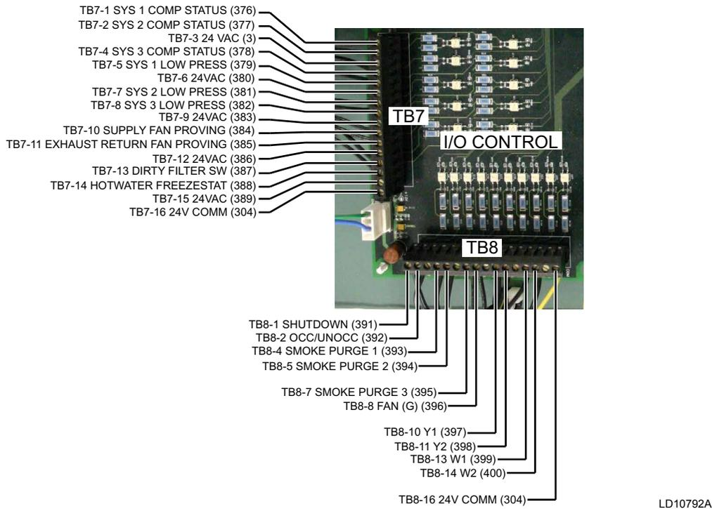
FIGURE 52 - I/O CONTROL BOARD - BINARY INPUTS
